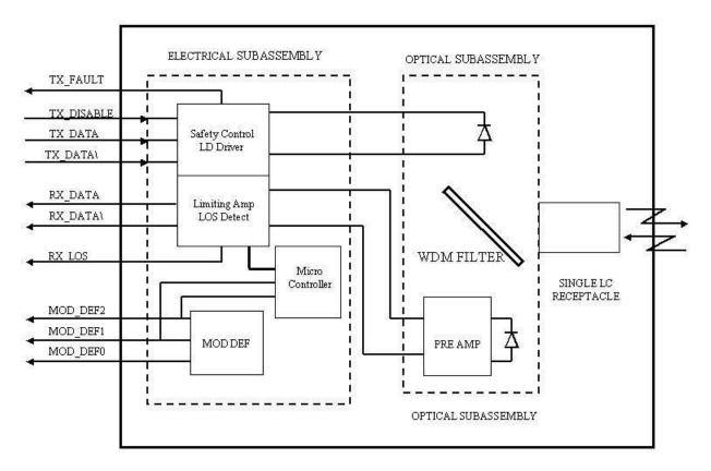
**Block Diagram of the Transceiver**
