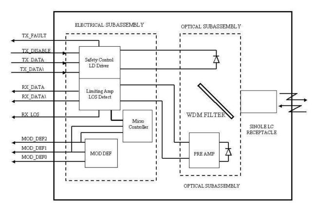
**Block Diagram of the Transceiver**
